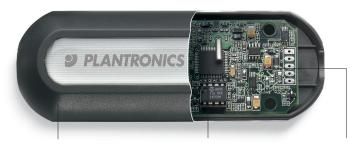
32-bit DSP modifies and enhances the audio signal for superior stereo sound and higher speech recognition accuracy. 24-bit high signal-to-noise ratio audio CODEC converts digital signal to enhanced analog sound for the highest quality PC audio. Digital circuitry matched to headset speakers and mic for maximum sound clarity.
