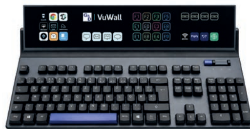
The keyboard executes control tasks without requiring a central server
